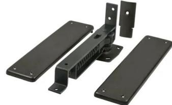
The Double Action Spring Hinge is a floor-mounted self-closing hinge with solid brass cover plates and trim. It swings in both directions and has a hold open feature at approximately 90 degrees.
