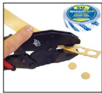
1. Apply SpeedTape to edgebanding
