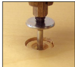
3. Countersink PowerHead screw
