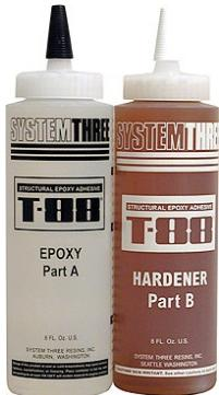
**Recommended uses:** For well over 25 years T-88 has been the most widely used structural adhesive for marine and general woodworking use in the U.S. Mixed at 1:1 by volume ratio, T-88 will cure at temperatures as low as 35° F. When fully cured, it is unaffected by water, oil, kerosene, and many other chemicals. It will not stain wood and is immune to fungus and rot. T-88 is unique in that it may be applied to damp wood, provided it is worked well into the surface.
