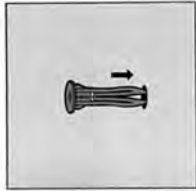
2. Insert anchor in 5/16" hole and tap flush with wall.
